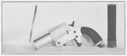
VERY SIGNAL PISTOL, WITH CARTRIDGE. FOR USE FROM AIRPLANE FOR COLORED FLASH SIGNALS, ETC.
